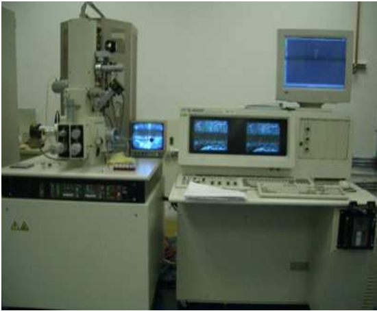
Figure II.13: MEB standard Philips XL30
