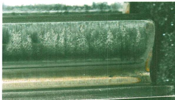
**Figure I.7 :** Le grippage "Engrenage".
