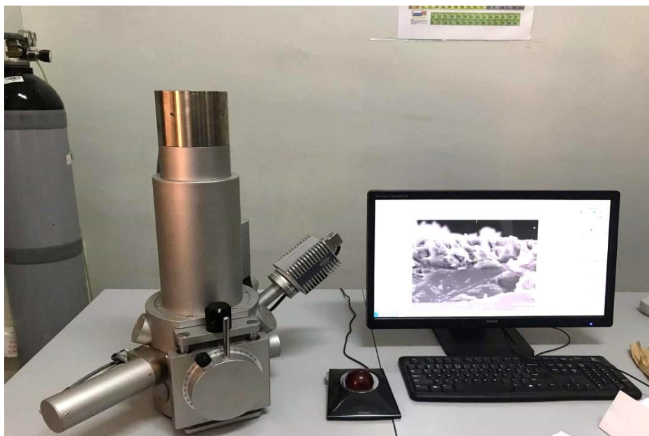
Figure II.11 Appareil MEB de type TESCAN VEGA3.
