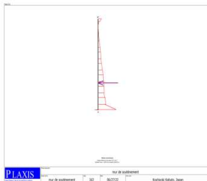
Figure V.15 : diagramme des contraintes effectives horizontales ( \sigma_{hmax}' = -93,3 \text{ KN/m}^2 )
