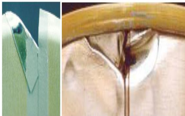
Figure I.12: Coin replié (ASMA, 2021).
