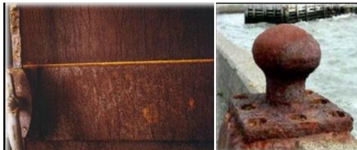
Figure II.6: Corrosion uniforme (Uhlig ,1970).
