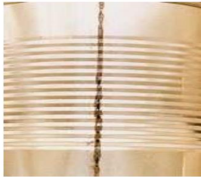
Figure I.11: Soudure brûlée (Lefaux, 1947)
