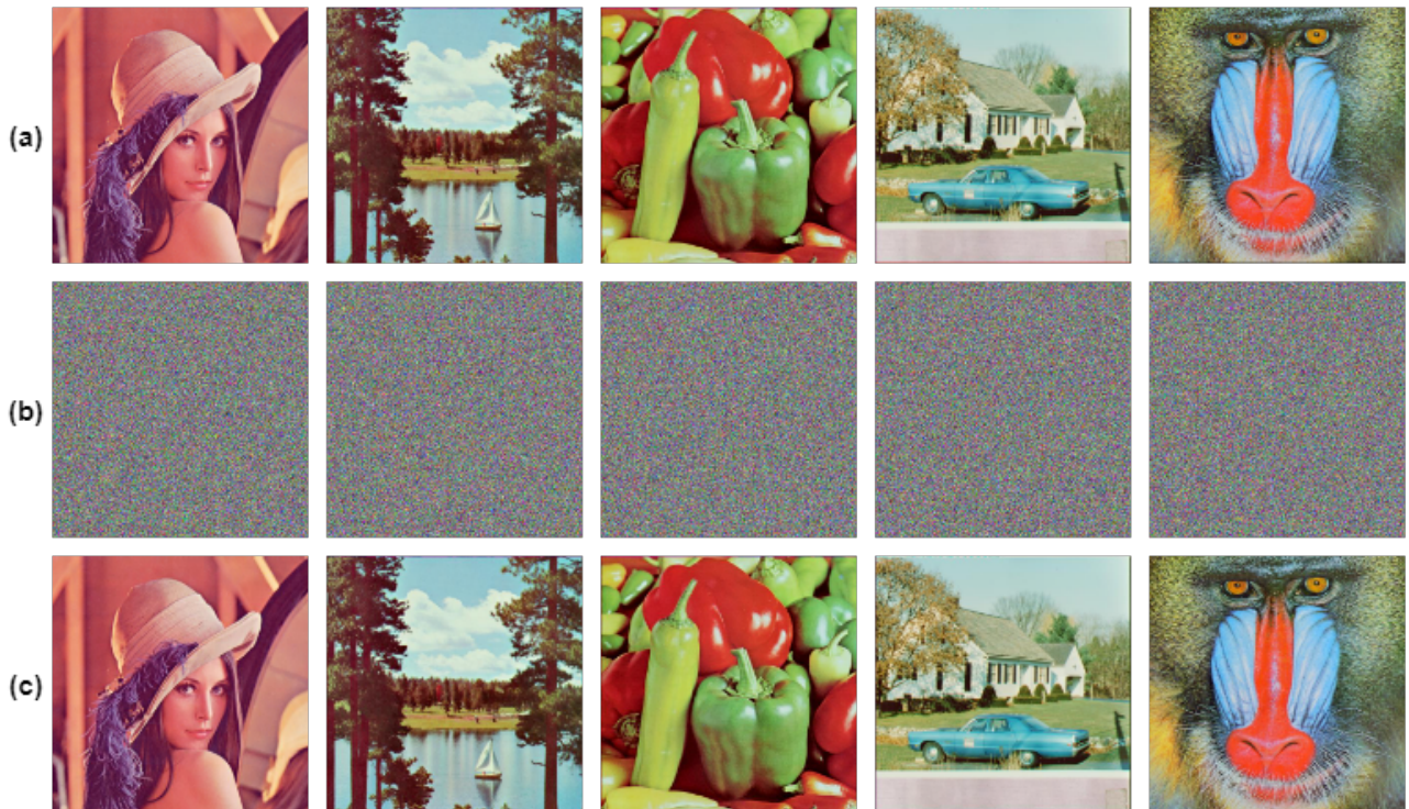
Figure 3.4: plain images encrypted and decrypted with the explained steps. (a) The original plain images. (b) shows the effects of the encryption. (c) is the decryption of the ciphered images.
