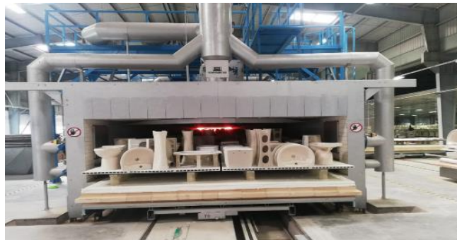
Figure 58: Firing at 1230 °C in an industrial tunnel kiln.
