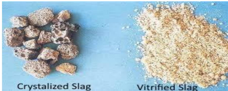
Figure 20: Blast furnace slag, crystalized and vitrified [54].
