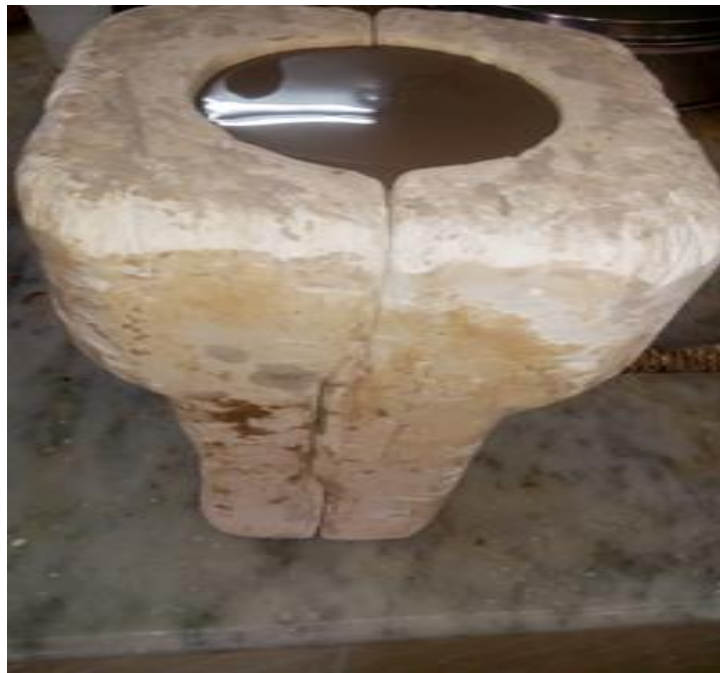
Figure 12: slip casting in plaster molds.
