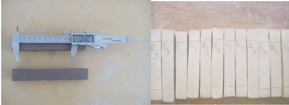
Figure 33: Example of green and fired ceramic bars for shrinkage and flexural testing.
