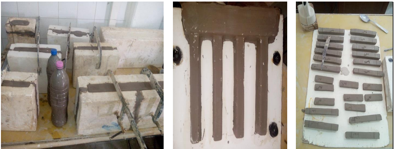
Figure 56: Casting slip into the plaster mould and re-emptying the slip.
