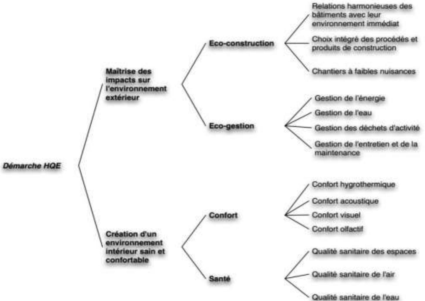
Figure 35: les cible HQE (source :INPL\_2011\_GHOLIPOUR\_V.pdf p
