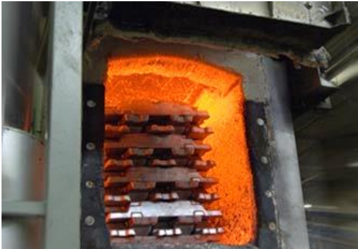
Figure II.15 : Processus de fusion [3].
