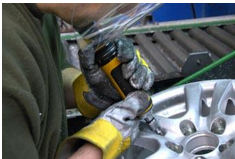
Figure II.21 : Ebavurage et finition de la jante [3].
