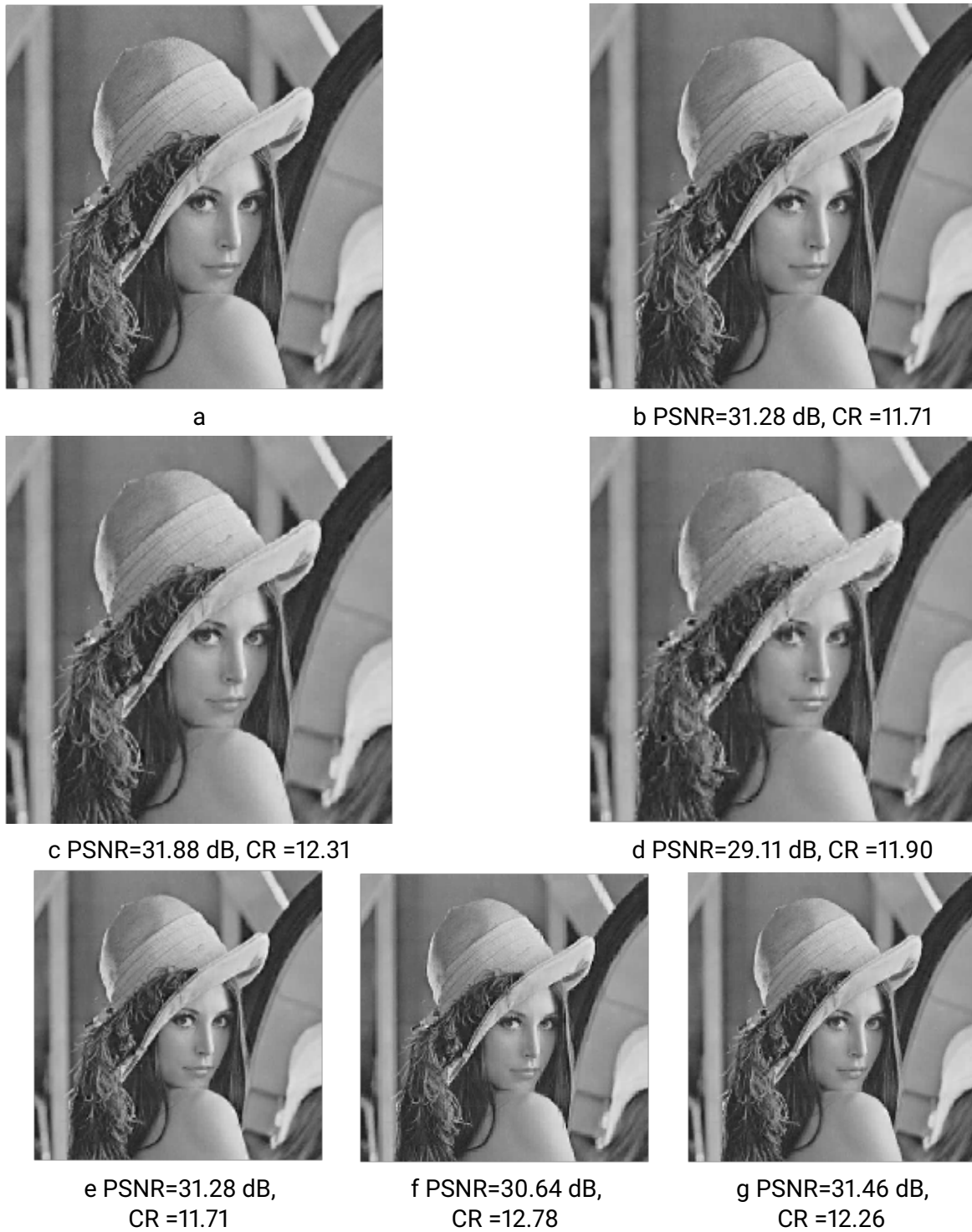
Fig. 4.15: The reconstructed Lena image using various transforms: (a) Original image, (b) Scaled DCT, (c) T_{10} , (d) T_{12} , (e) T_{14} , (f) T_9 , (g) T_{p4}
