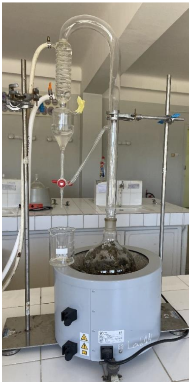
Figure 18: Hydrodistillation of Mentha rotundifolia essential oils Clevenger-type Apparatus
