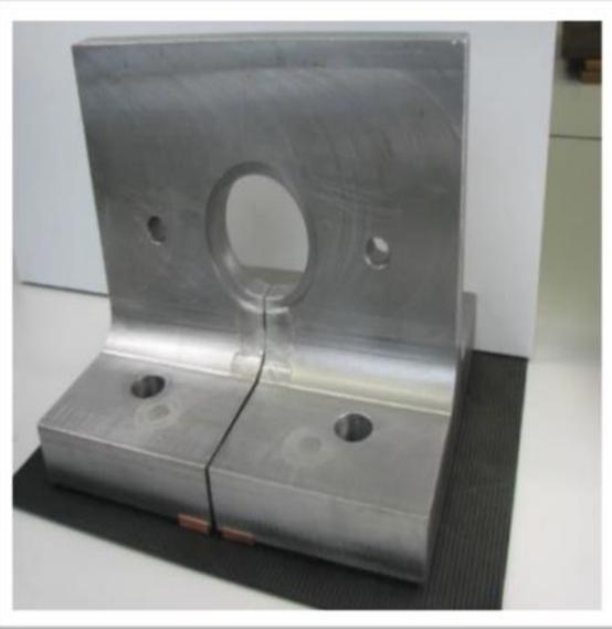
**Figure I.11 : Bobine à un seul tour**
