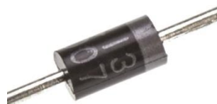
Figure I.19. Diode de redressement type 1N4007
