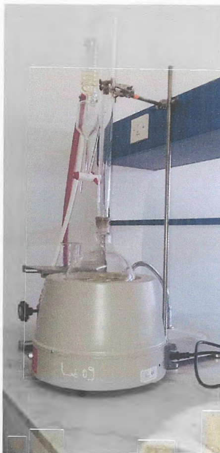
Figure 8: Hydrodistillation of Essential Oils: Clevenger-type Apparatus Materials.
