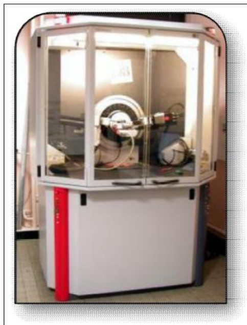
Figure II.5: Image d'un diffractomètre Bruker D8 Advance.
