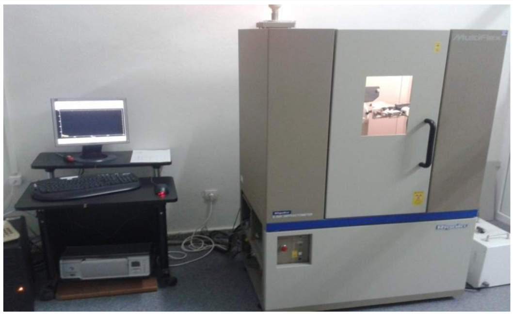
Figure. II.3: Diffractomètre des rayons X de type D8 Advance Bruker AXS.
