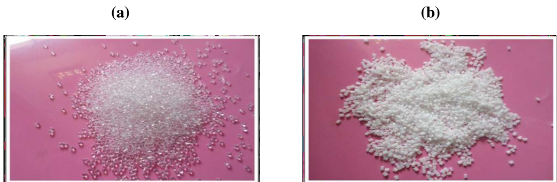
Figure I.2: (a): Le polystyrène cristal. (b):Le polystyrène choc.
