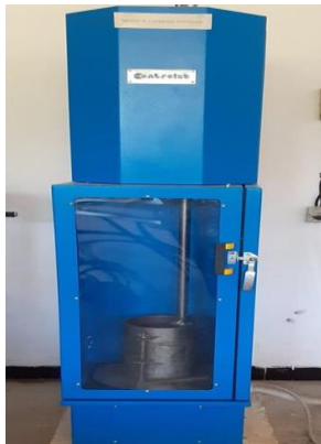
Machine de compactage
