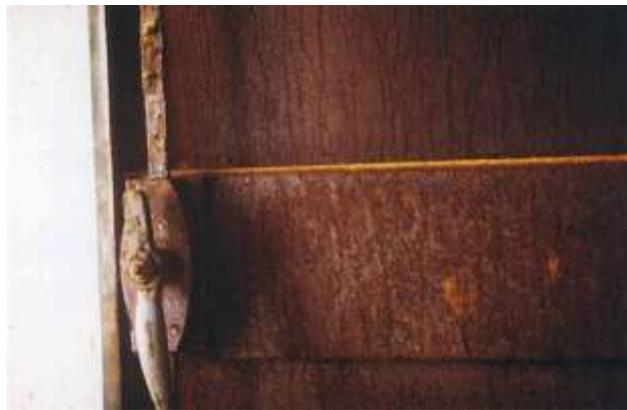
**Figure II.4 :** La corrosion uniforme.
