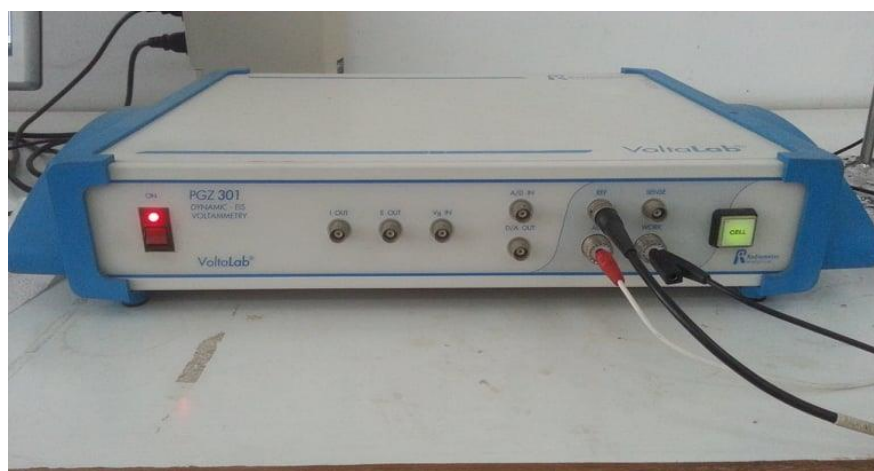
Figure II.8. Le potentiostat PGZ 301.
