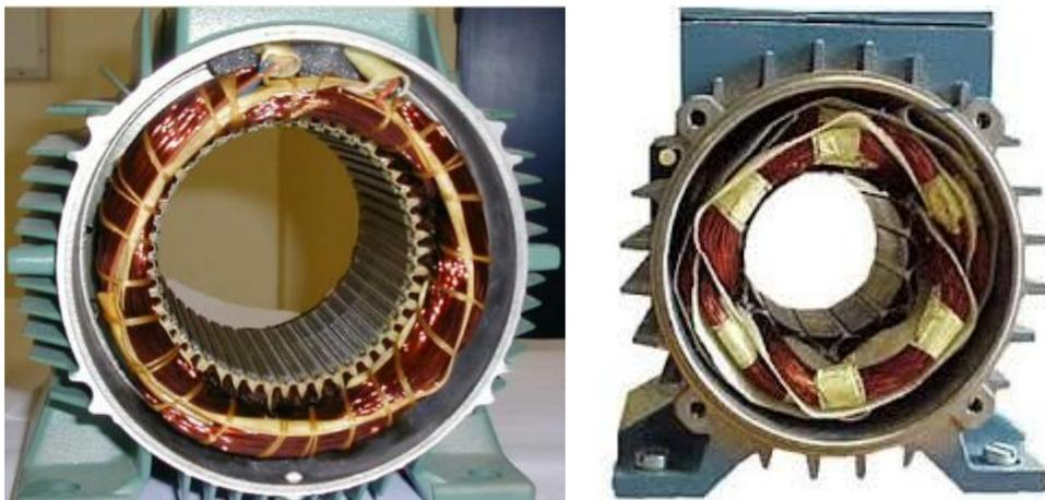
**Figure I.2 :** Le stator
