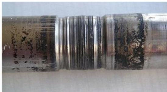
**Figure I.7.** Usure abrasive [19].
