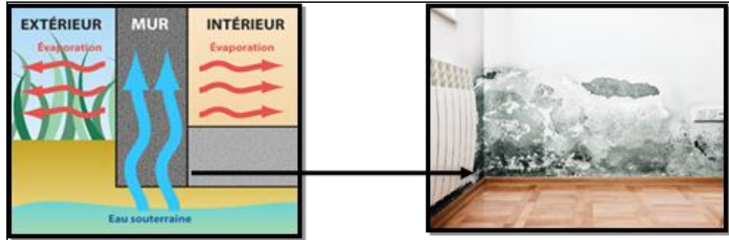
Figure [II.2] : la remontée capillaire
