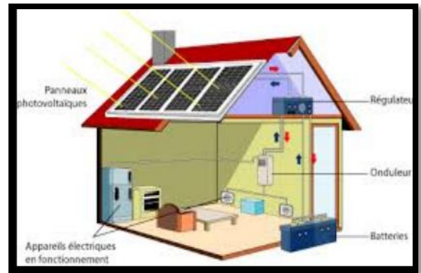
Figure34: installation solaire photovoltaïque
