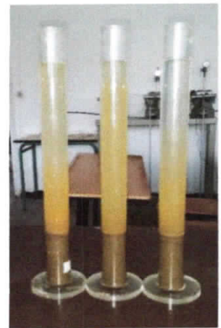
Figure (II.2) : Equivalent de sable.
