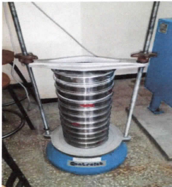
Figure (II.10) : Machine de tamisage.
