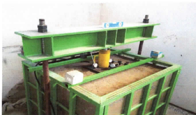
Figure (I.23) : la plaque de charge
