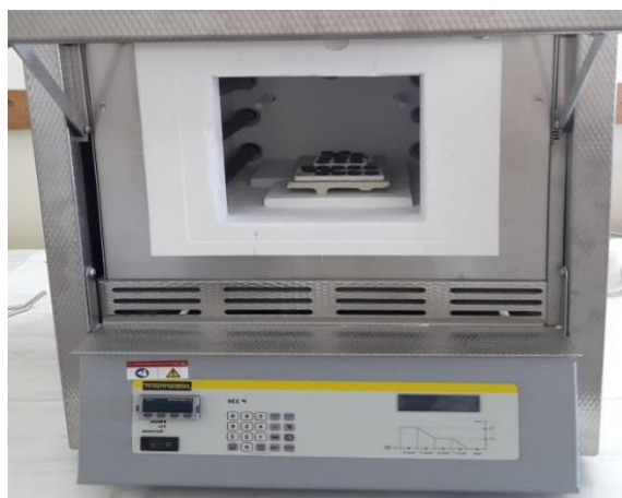
Figure II.3: Four de type Nabertherm .
