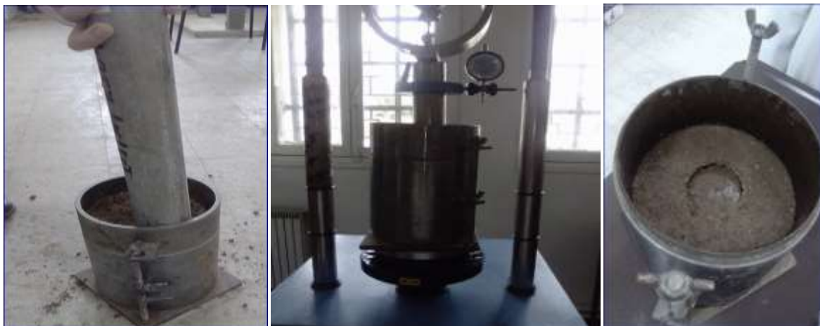
Figure III.19 :Appareillage de l'essai CBR
