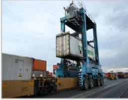
Circulate over container piles. Can go over stacks up to 3 in height. Density of 500 to 700 TEU per hectare.
